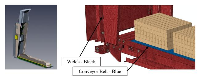
*FEA and Code Results*: With consideration to belt tension loading, dead-weight of equipment and luggage, along with evaluation of various inclination angles and opening/closing, the new chute was found acceptable for the required industry loads.
